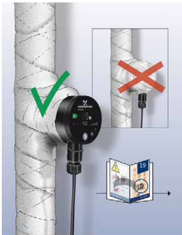
Fig. 5 Insulation of pump housing
