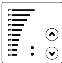
Fig. 21 Control panel of a CME pump
