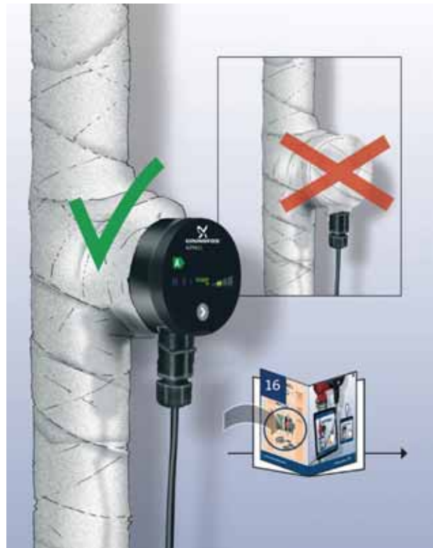
Fig. 5 Insulation of pump housing
