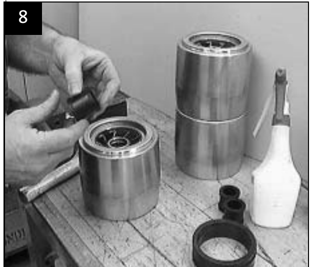
Fit rubber bearing in chamber
