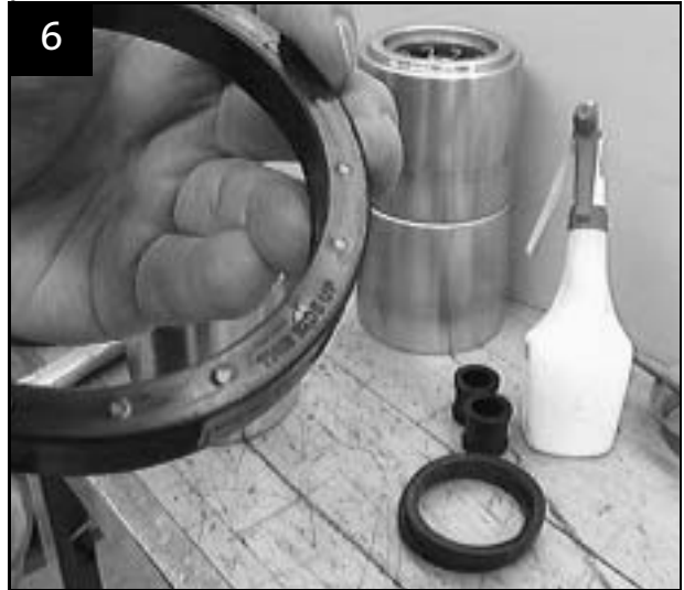
'THIS SIDE UP' must point upwards
