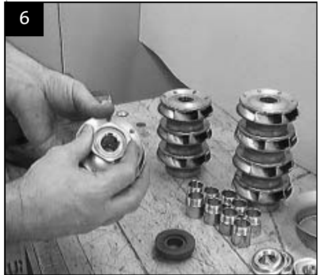
Fit split cone and split cone nut in impeller
