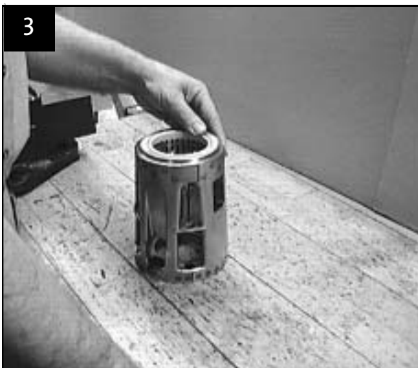
Strainer and bottom neck ring fitted in suction interconnector
