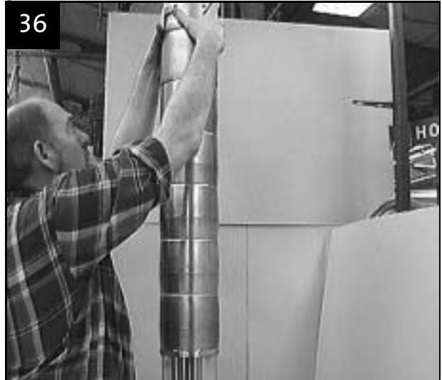
Fit valve casing
