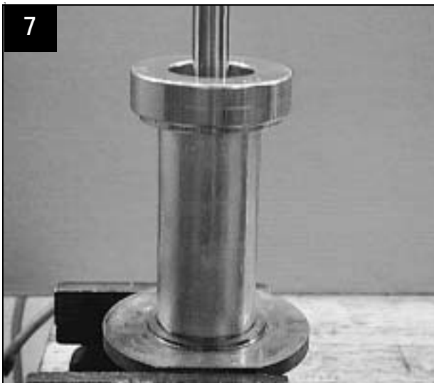
Shaft with coupling in assembly tool
