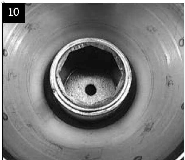
10 Fit upthrust bearing in top chamber. Continued on page 18.
