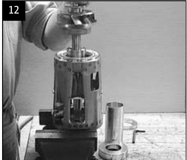
Fit shaft with impeller in suction interconnector
