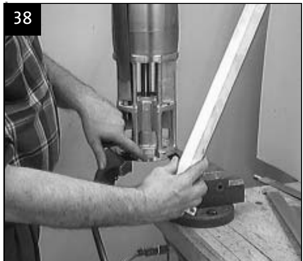
Position of cable guard in suction interconnector and in valve casing must be aligned
