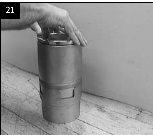
21 Fit retainer in valve casing
