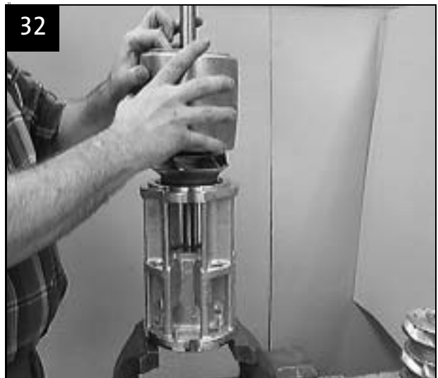
Fit bottom intermediate chamber stop ring
