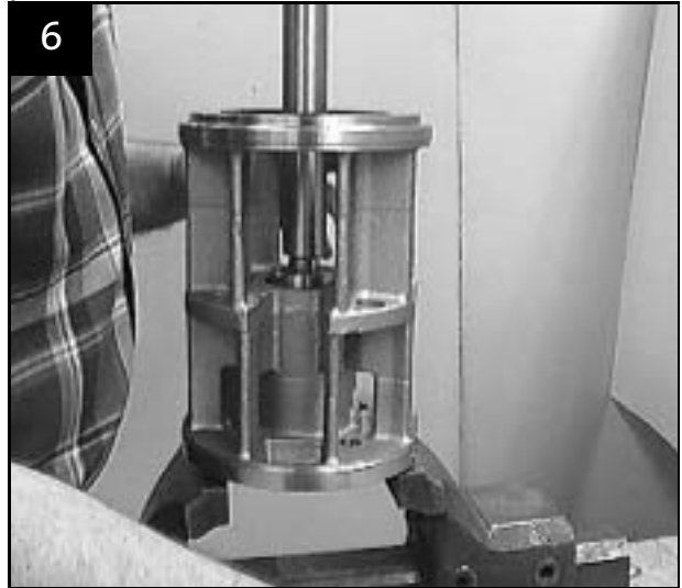
6 Fit shaft loosely in suction interconnector to make the impeller centre the shaft
