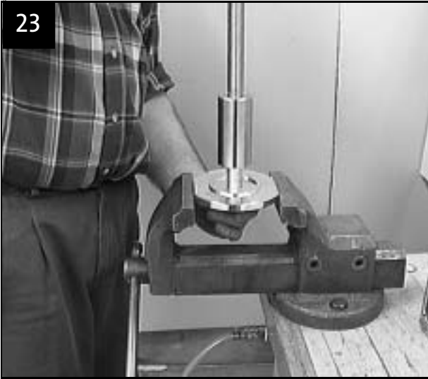
Pump shaft with coupling in assembly tool
