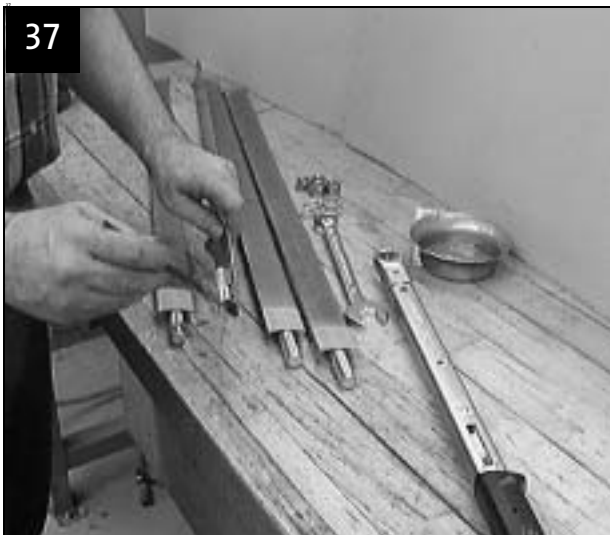
Lubricate threads with Bonderlube
