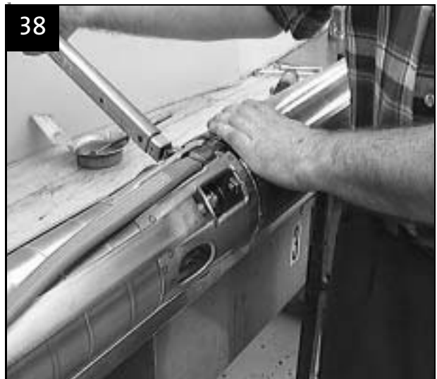
Tighten motor bolts
