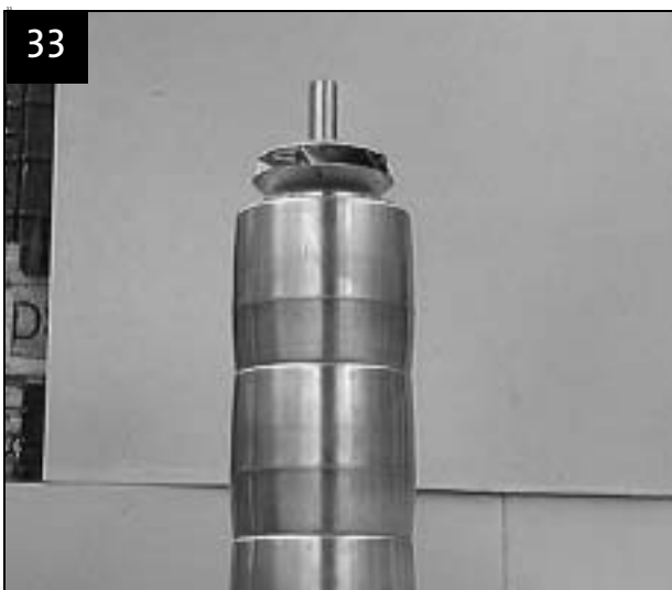
All impellers and chambers fitted
