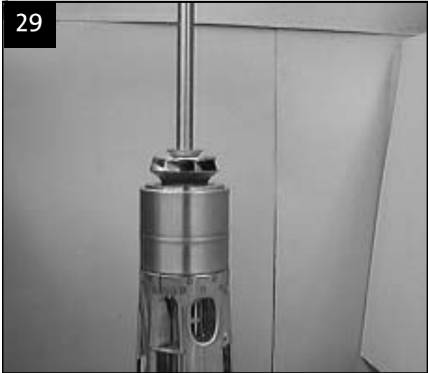
Chamber with stop ring fitted
