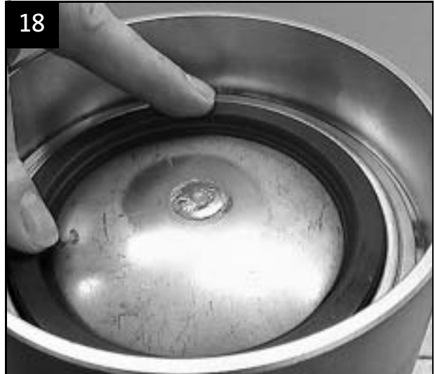
18 Fit neck ring in valve casing
