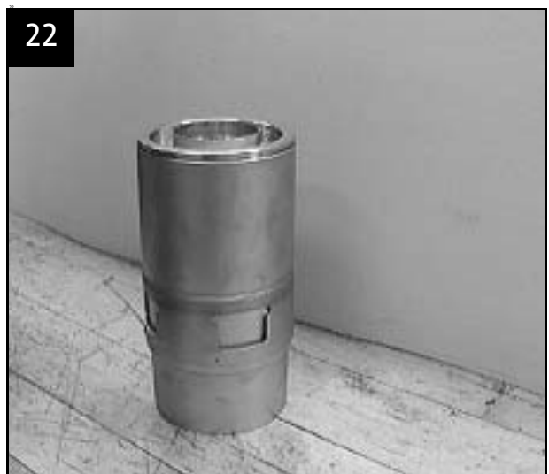
22 Valve casing completed
