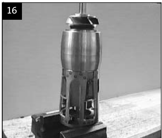
Bottom chamber and impeller fitted. Continued on page 18.
