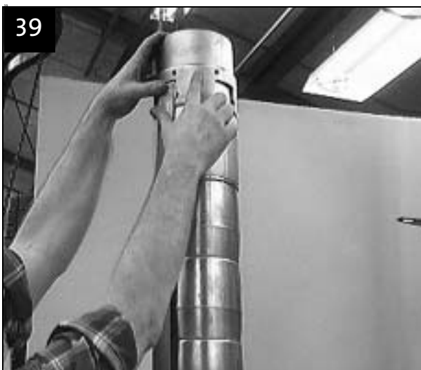
Position of cable guard in suction interconnector and in valve casing must be aligned
