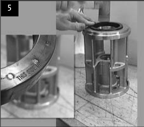
5 Fit neck ring in suction interconnector. 'THIS SIDE UP' must point upwards
