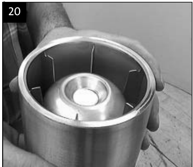
Valve casing with non-return valve
