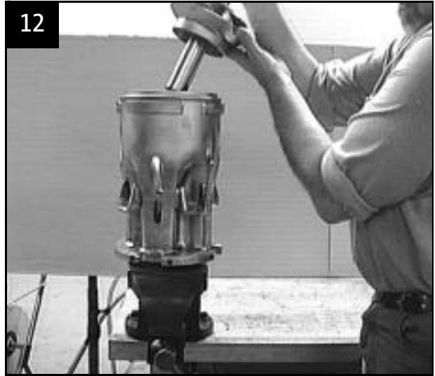
Fit shaft with impeller in suction interconnector
