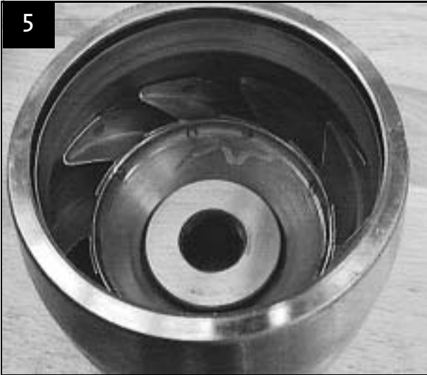
Stationary stop ring fitted in chamber
