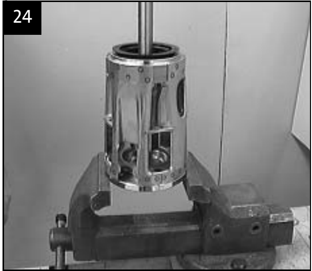
Suction interconnector fitted
