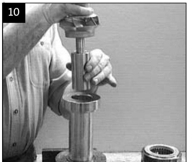
Remove shaft and impeller from assembly tool
