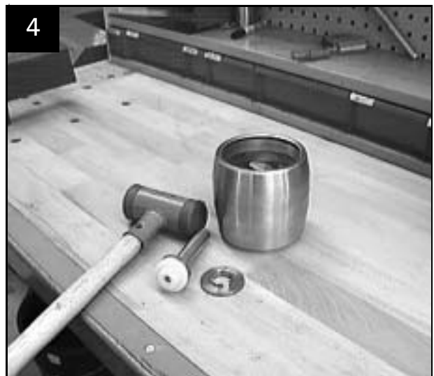
Fit stationary stop ring in chamber
