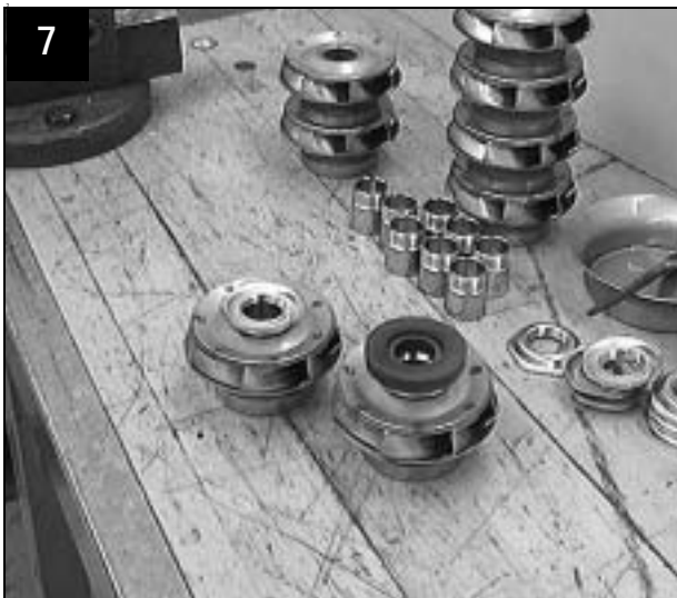
Spacing washer for stop ring placed on first impeller
