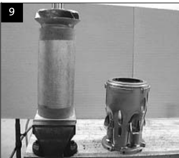
Mounting pipe and suction interconnector (to be reversed)
