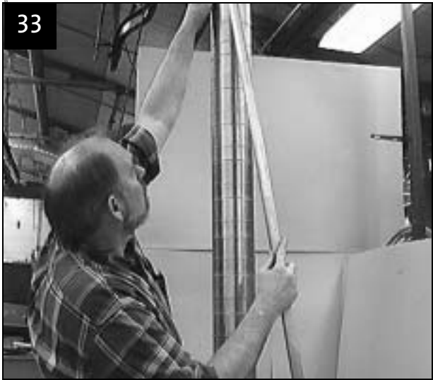
Fit straps on pump cylinder
