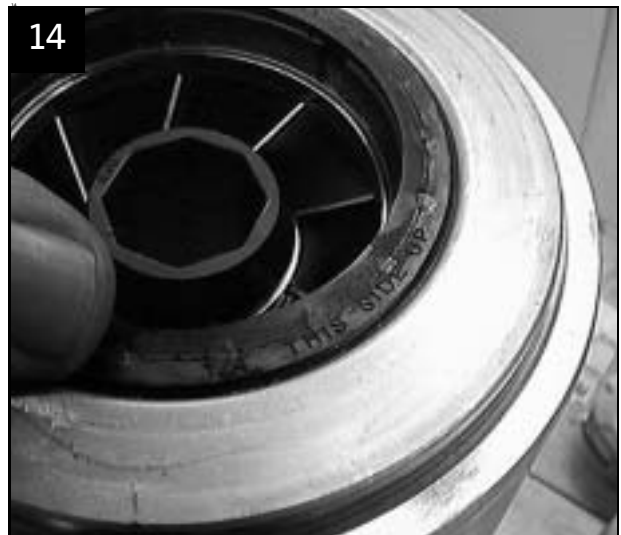
'THIS SIDE UP' must point upwards
