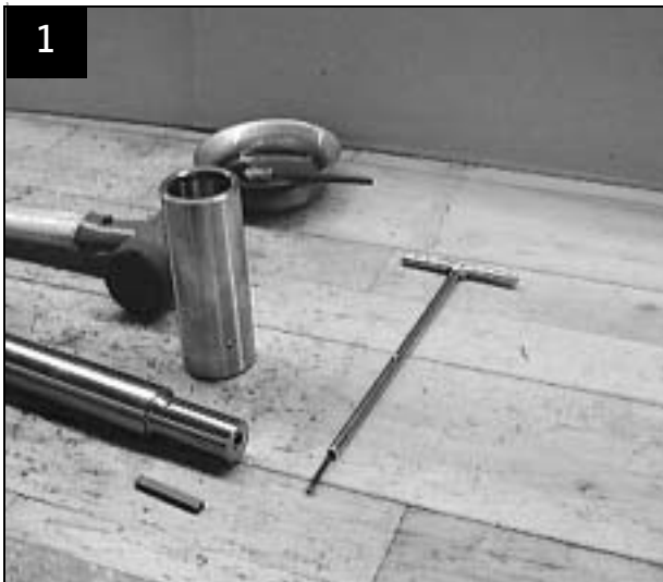
Fit coupling and key on shaft
