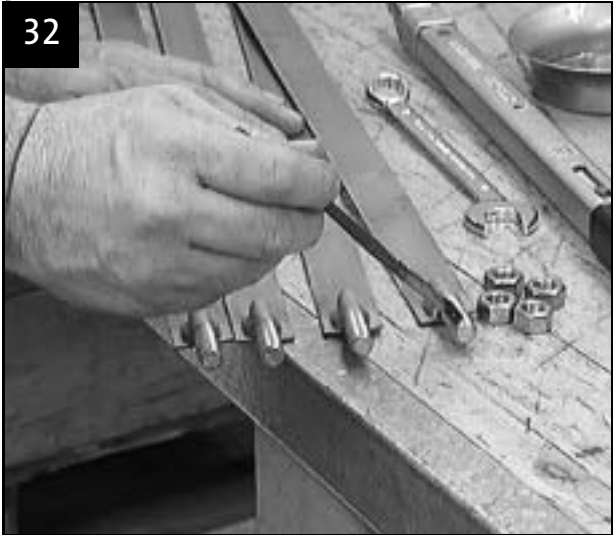
Lubricate threads with Bonderlube
