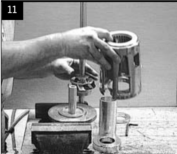
Mount suction interconnector on assembly tool
