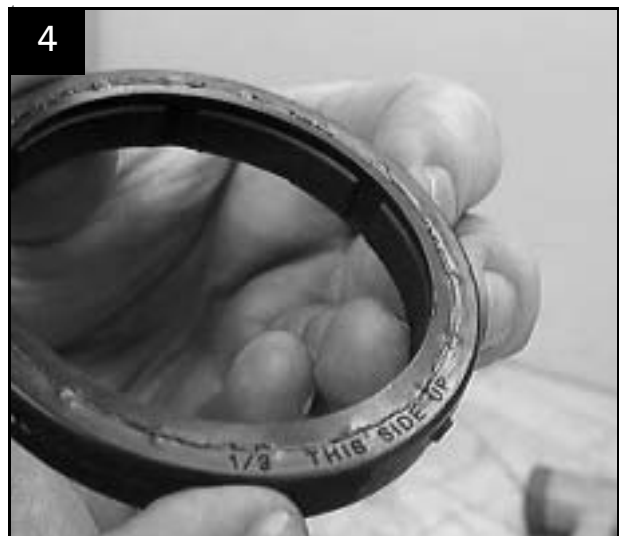
'THIS SIDE UP' must point upwards
