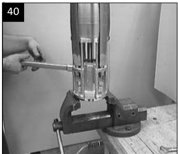
Tighten strap nuts at specified torque
