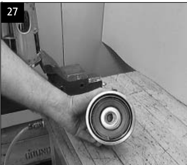
Spacing washer for stop ring fitted
