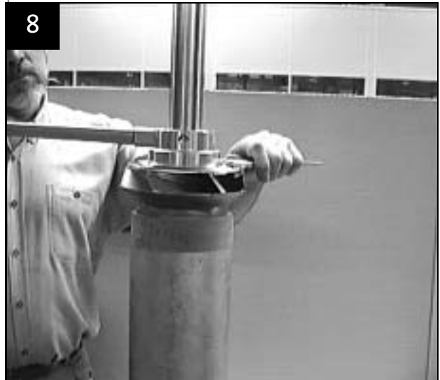
Tighten first impeller
