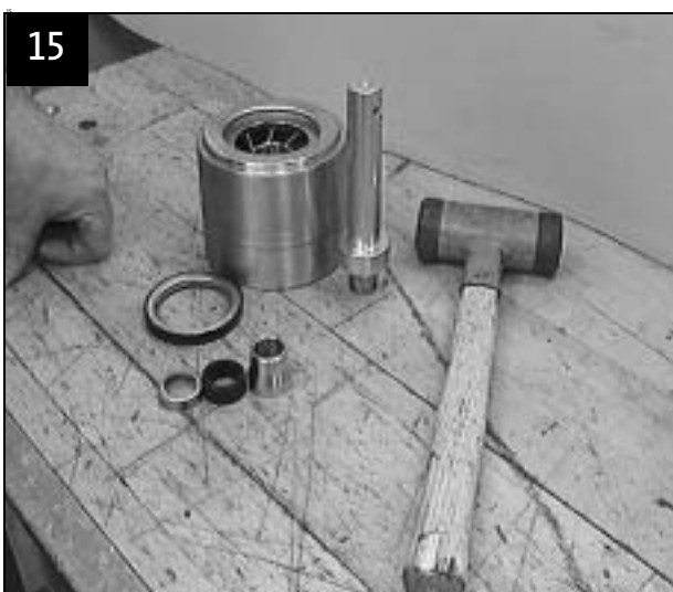
Fit top bearing in top chamber
