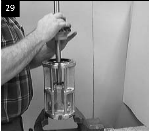
Fit first impeller including stop ring
