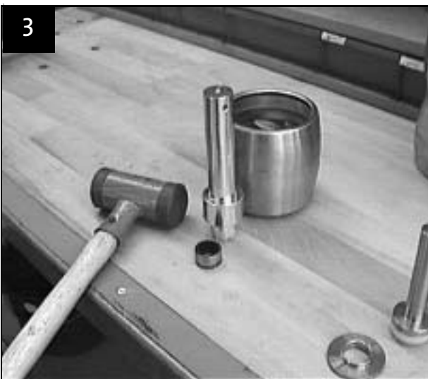
Fit lower bearing in chamber
