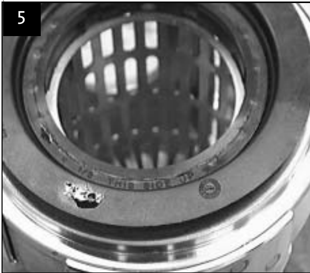
Neck ring fitted correctly in suction interconnector
