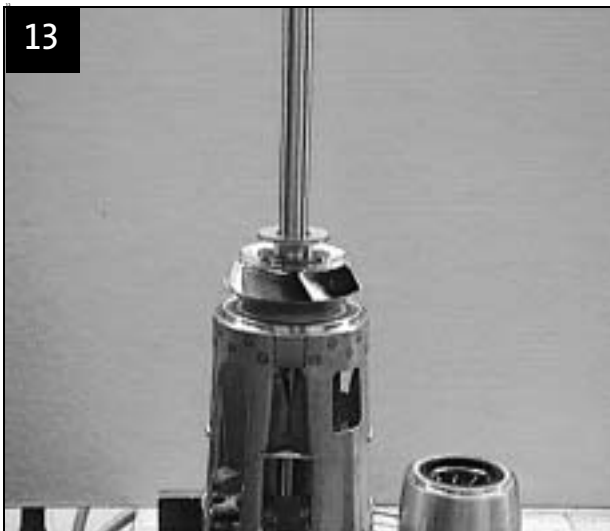
Shaft with impeller fitted in suction interconnector
