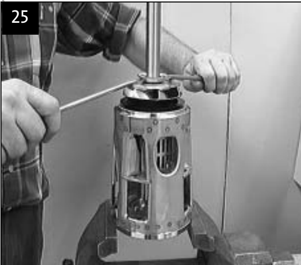
Fit first impeller
