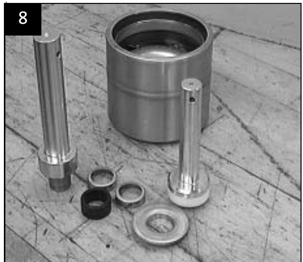
Intermediate bearing and upper stop ring including tools
