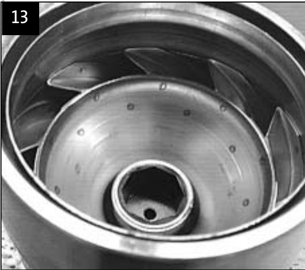
Fit upthrust bearing in top chamber. Continued on page 18.
