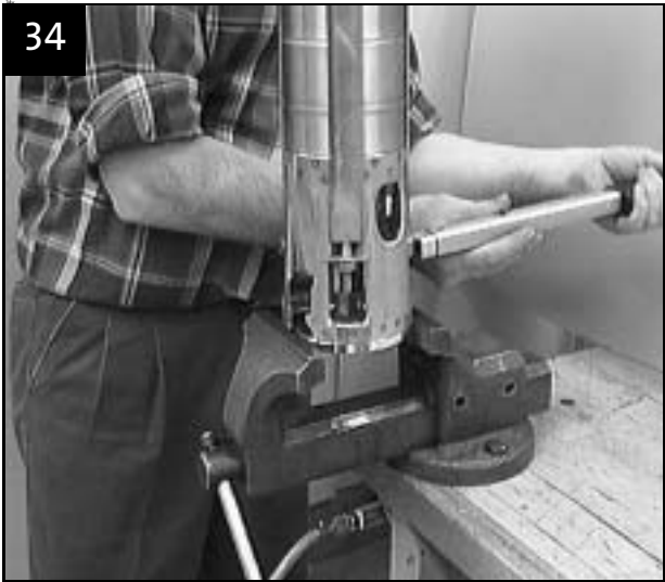
Tighten strap nuts at specified torque
