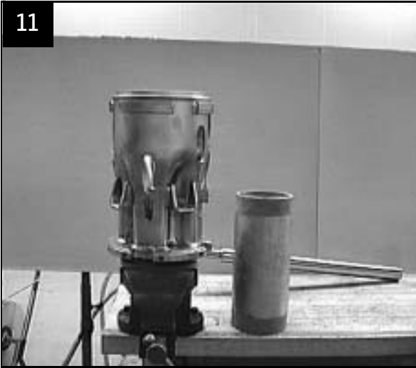
Replace mounting pipe with suction interconnector
