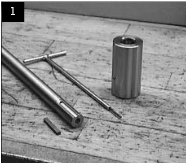
Fit key and coupling on shaft
