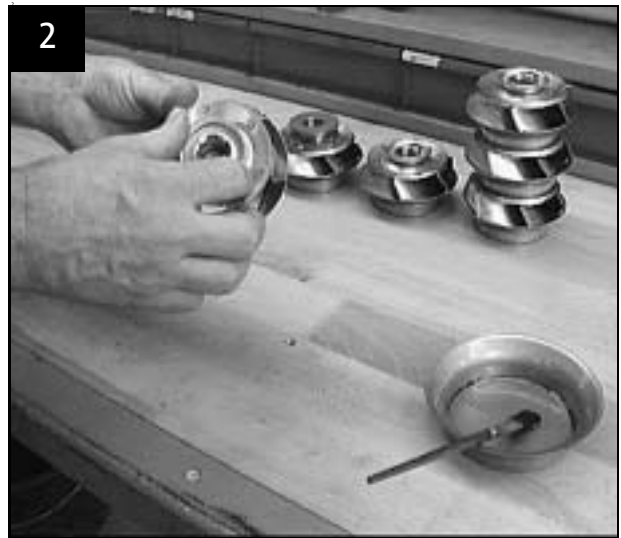
Split cone and split cone nut fitted in impeller
