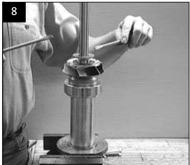
Fit first impeller including stop ring
