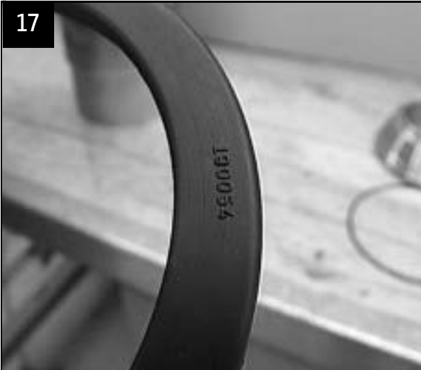
17 The side of the rubber ring with the numbers must point upwards
